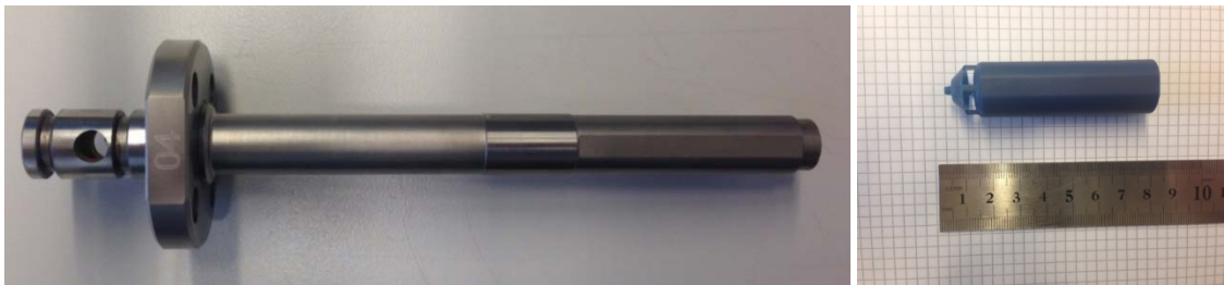
Figure 1: left: Cylindrical insert that has been surface treated and tested in an injection mould right: Test piece. Several polymers that are commonly in use in plasturgie have been tested.
